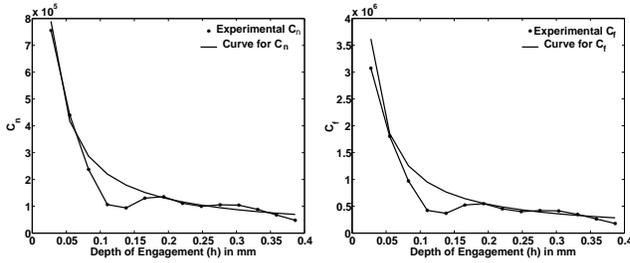
FIGURE 9: THE VARIATION OF  $C_n$  AND  $C_f$  WITH  $h(i)$  AT 250 RPM.
