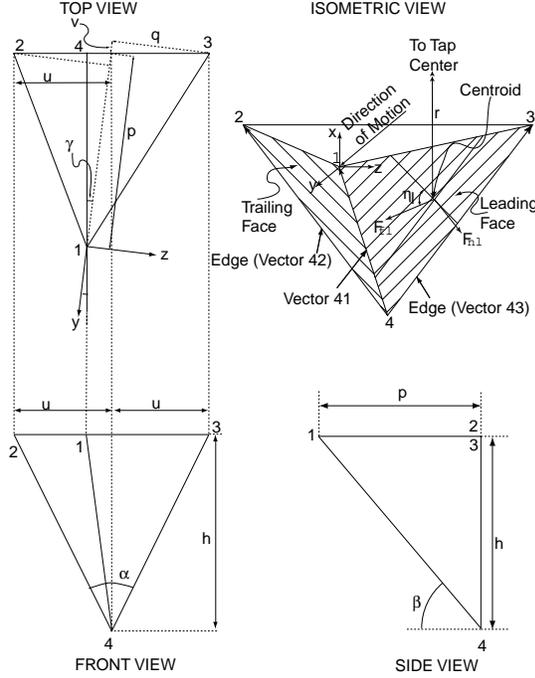
FIGURE 6: GEOMETRY OF A SINGLE TAP TOOTH.
