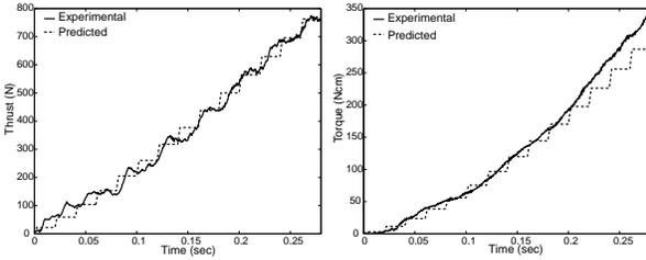
FIGURE 12: PREDICTED AND EXPERIMENTAL VALUES OF THRUST AND TORQUE IN THE MODELED REGION AT 750 RPM.
