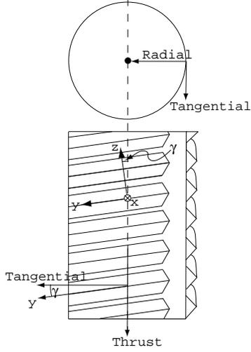
FIGURE 8: TRANSFORMATIONS FROM TOOTH TO TAP COORDINATES.
