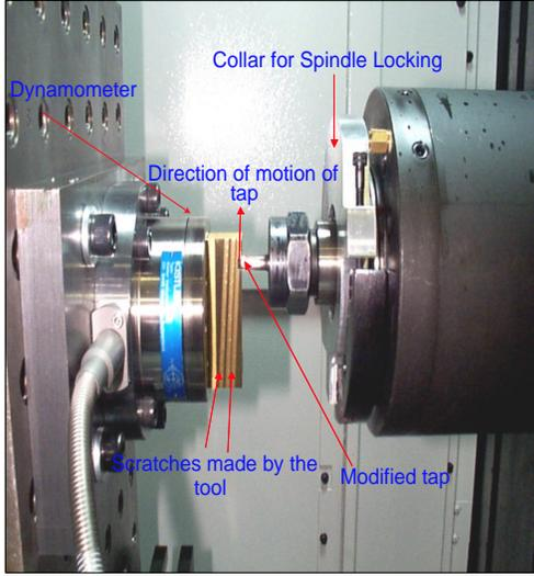
FIGURE 3: THE EXPERIMENTAL SETUP FOR TOOTH-LEVEL EXPERIMENTS.
