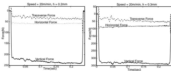
FIGURE 5: THE FORCES AT  $h = 0.2$  mm AND  $h = 0.3$  mm FOR 20 m/min SURFACE SPEED.
