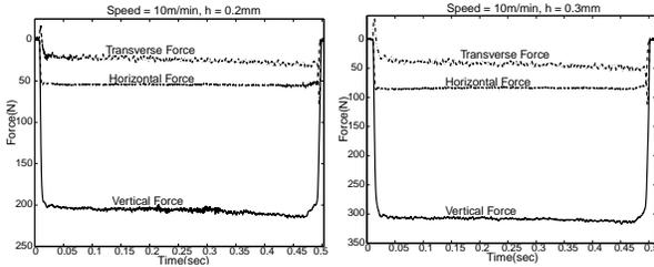
FIGURE 4: THE FORCES AT  $h = 0.2$  mm AND  $h = 0.3$  mm FOR 10 m/min SURFACE SPEED.
