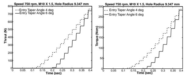
FIGURE 15: PREDICTED THRUST AND TORQUE VALUES FOR DIFFERENT ENTRY TAPER ANGLES.
