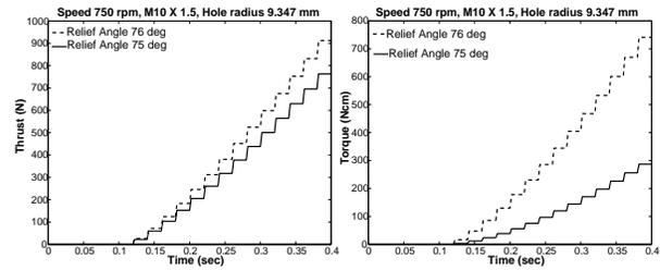
FIGURE 14: PREDICTED THRUST AND TORQUE VALUES FOR DIFFERENT RELIEF ANGLES.
