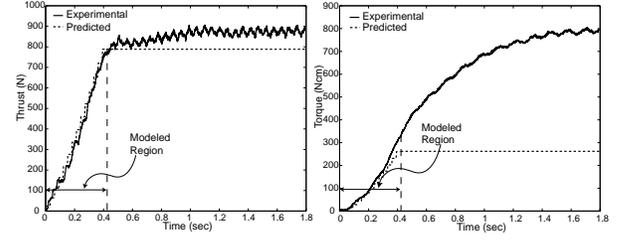
FIGURE 10: PREDICTED AND EXPERIMENTAL VALUES OF THRUST AND TORQUE AT 500 RPM.
