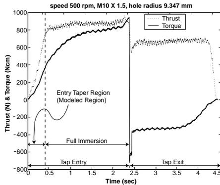
FIGURE 13: EXPERIMENTAL FORCES DURING A TYPICAL FORM TAPPING OPERATION.
