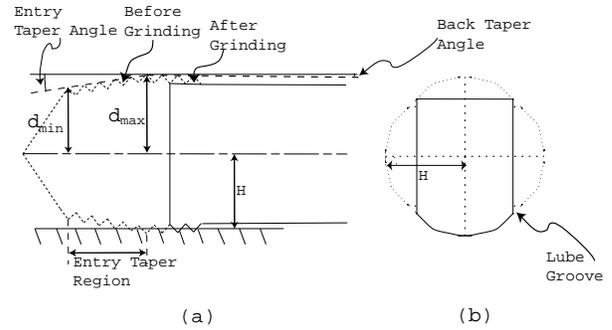
FIGURE 1: (a) FORM TAP; (b) CROSS-SECTION OF A FORM TAP.
