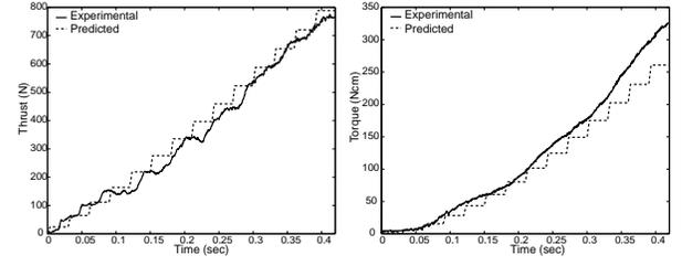
FIGURE 11: PREDICTED AND EXPERIMENTAL VALUES OF THRUST AND TORQUE IN THE MODELED REGION AT 500 RPM.
