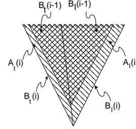
FIGURE 7: THE AREAS OF CONTACT OF THE  $i^{th}$  TOOTH.
